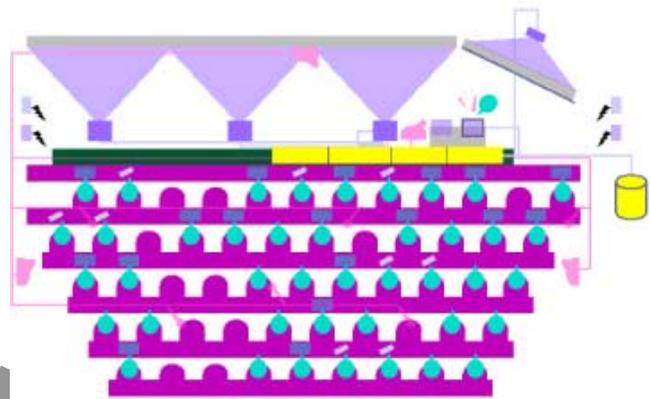
Fig. 4: Schematic drawing of a DLH configuration with Smartboard™, beamer array, and Pen-LCD-Tablet (purple, upper part); server and recording hardware (yellow); PTZ cameras and microphones (light pink); wLAN / PAN network and learner appliances
