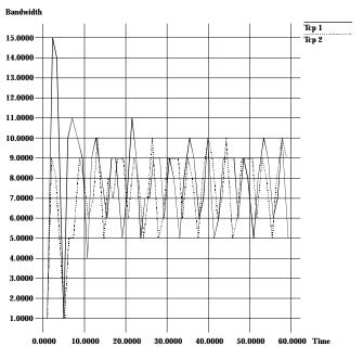
Fig. 8: Bandwidth / time plot of two TCP sources sharing the same bottleneck with RED queueing
