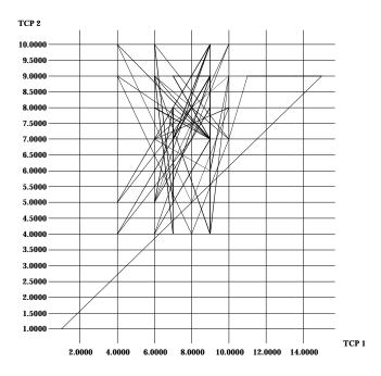
Fig. 5: Vector diagram of two TCP sources sharing the same bottleneck with DropTail queueing
