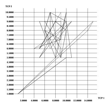
Fig. 6: Vector diagram of two TCP sources sharing the same bottleneck with RED queueing
