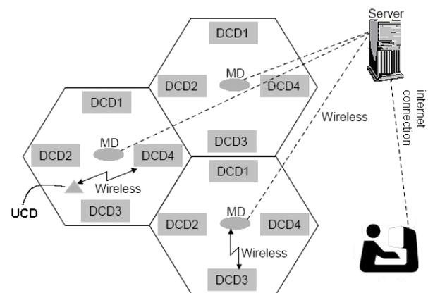
Figure 1: The Network Topology for the ubiquitous computing
