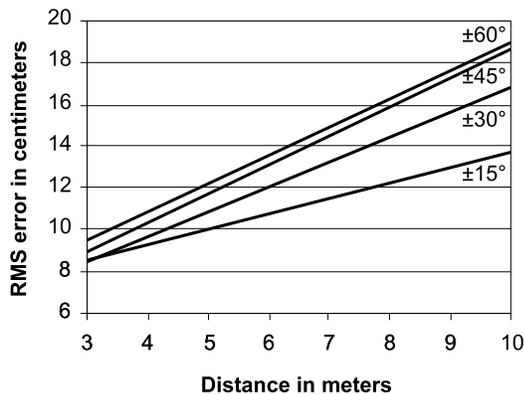
Figure 4: Root Mean Square accuracy of the IRIS tracking system as a function of distance and opening angle.
