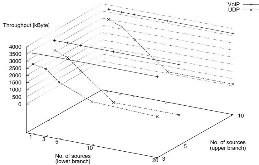
Figure 7. Throughput of a setup with and without using VoIP proxies
