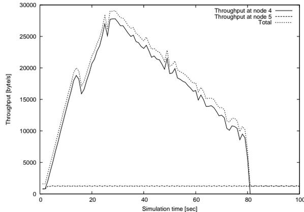
Figure 2. Congestion collapse caused by 2 UDP/CBR sources
