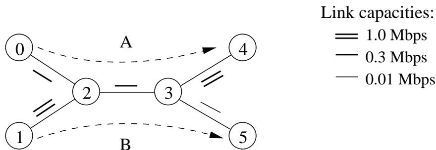
Figure 1. Congestion collapse test topology (Dumbbell)
