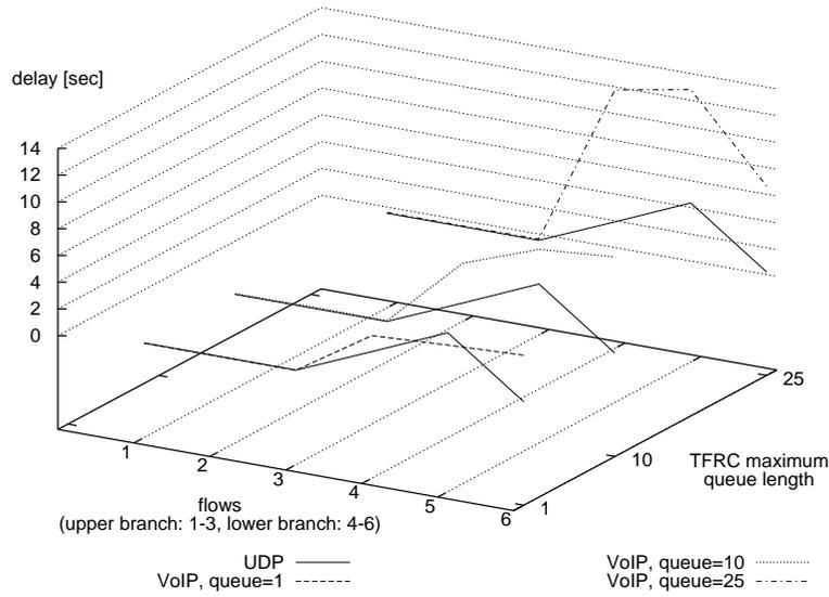
Figure 6. Mean one-way delay subject to the TFRC maximum queue length
