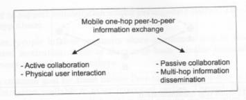
Fig. 25.2: Design space of mobile one-hop Peer-to-Peer communication
