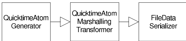
Figure 3. Pipeline of SABRE StreamHandler components used for the generation of Apple QuickTime movies
