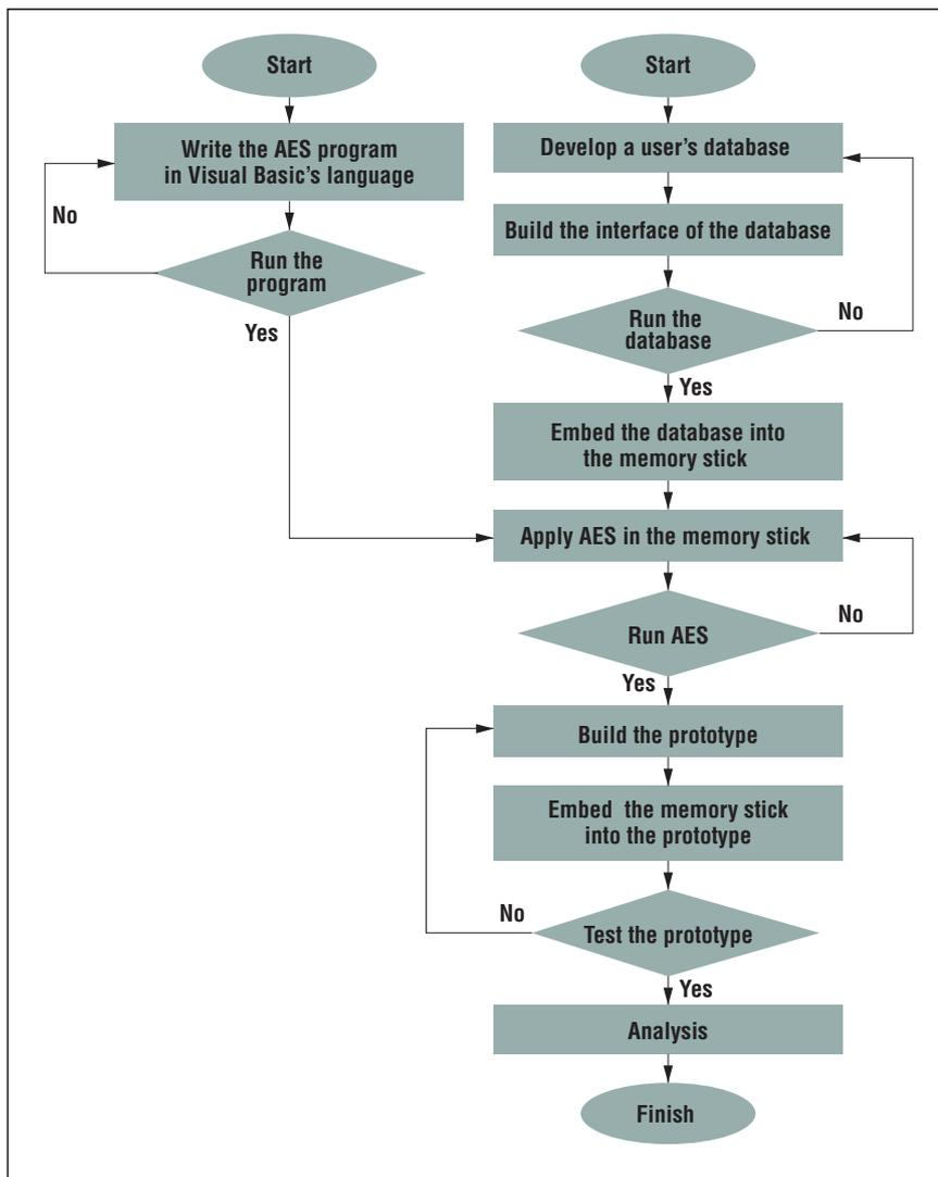
Figure 2. Steps taken in developing the e-passport application.
