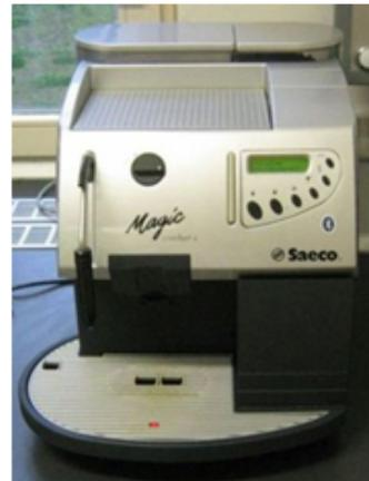
**Fig. 5** A coffee machine turned into a smart product. Sensors and communication electronics were added inside the machine's case.
