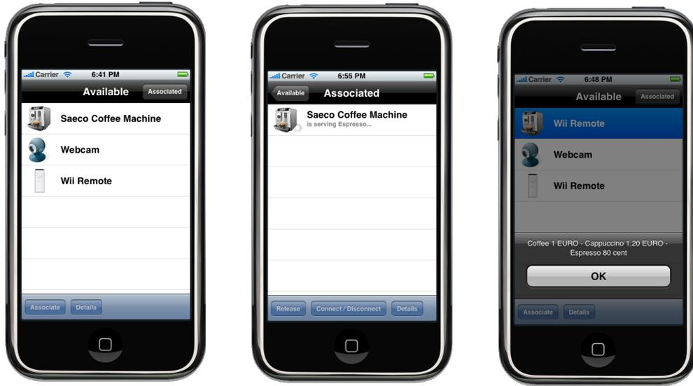
**Fig. 4** Screenshots of the MINE manager interface running on the iPhone as an example of a *personal trusted device*. The left screen shows the list of available  $US/P_{dig}$  in the LAN zone. The middle screen shows the associated  $US/P_{dig}$  in the MINE. The right screen shows the details for a single smart product.
