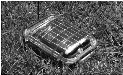
Figure 1. A solar harvesting sensor node (Heliomote [2])
