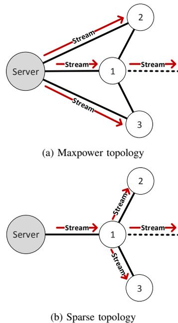
Fig. 1: Two underlay topologies with overlay streaming routes
