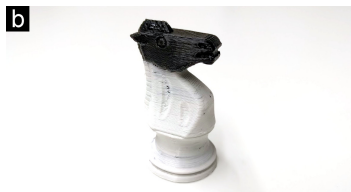
Figure 4: (a) Two sets of 3D printed chess pieces, and (b) a single knight. White parts are made of regular plastic, black parts are made of conductive material.
